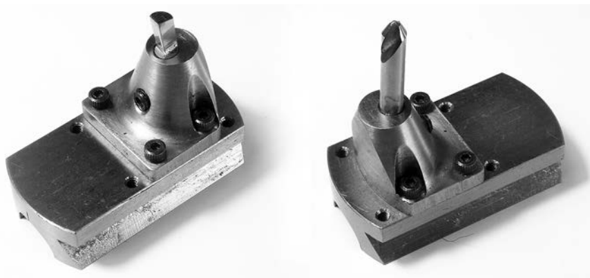
Figure 1.7: The tool holder, and (right) showing a broken BS2 centre drill from which the tool bit can be ground
